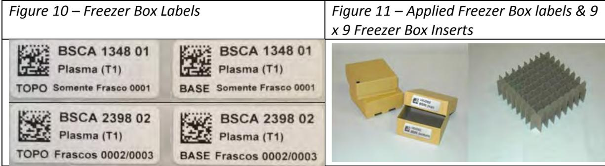
All 2 mL cryovials should be stored in standard 2” specimen boxes with a 9 x 9 insert (See **Figure 11**). The 9 mL Tempus tubes should be stored in 3” specimen boxes using a 7 x 7 insert.
